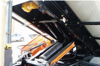
DC Truck Vibrator installed to maintain flow of frozen materials
