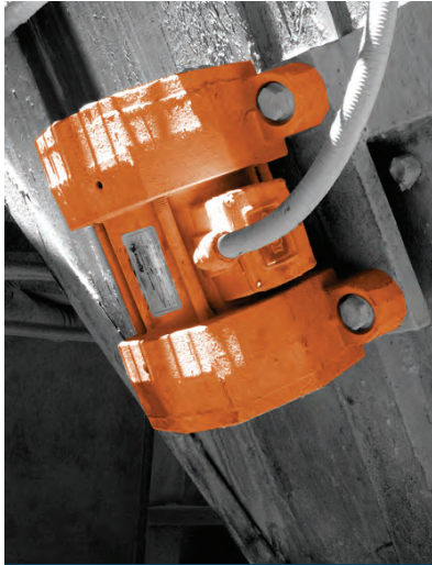
Electric Vibrator Mounted to Railcar Solves Unloading Problem
