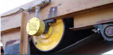
Motorized Pulley Reduces Costs in Corrosive Environment
