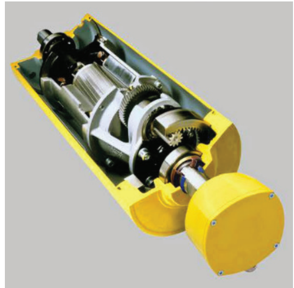
Figure 1. Motorized pulley with non-rotating drive train mounted on dead shaft within an oil-filled shell
