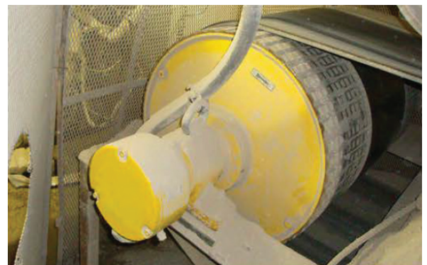
Figure 4. Motorized pulley installed in reclaim tunnel subject to flooding. Note partial lagging on outer thirds of pulley shell.
