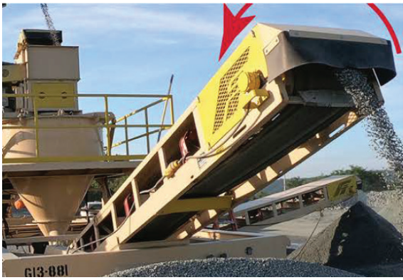
Figure 5. Motorized pulley transfers conveyor belt drive torque directly into structure, eliminating structural twisting during start-up
