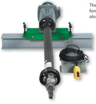
The **GO-E2** is an electric-powered Gate Opener with a rotating platform (for a full 360° swivel) on a rolling carriage (to mount and slide along a secured-to-ground W-beam), utilizing pendant-controlled, instant Forward-Reverse action, and a telescoping drive
