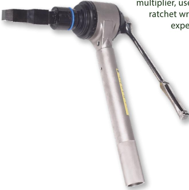
The **GO-M3** is a manual-powered, hand-portable, compact Gate Opener that rests on the ground when being used. The **GO-M3**, a heavy-duty torque multiplier, uses planetary gear action to enable an operator to simply turn a ratchet wrench to open gates. The **GO-M3** is well suited for worksites that experience:
