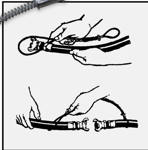
*Easily installed by depressing spring and looping the wire over the hose on both sides of the connection. Release the spring and the Whipcheck locks onto the hose creating a permanent, dependable safeguard.*
