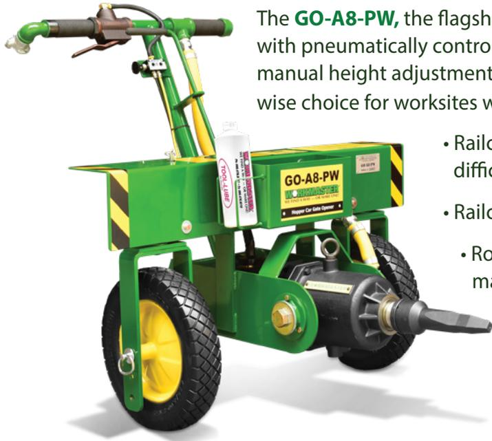
The **GO-A8-PW**, the flagship of our line, is an air-powered Gate Opener on a wheeled-cart with pneumatically controlled pivot wheels (to follow traveling gate or moving train), and manual height adjustment (accommodate varied-height capstans). The **GO-A8-PW** is the wise choice for worksites which experience:
