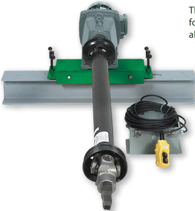
The **GO-E2** is an electric-powered Gate Opener with a rotating platform (for a full 360° swivel) on a rolling carriage (to mount and slide along a secured-to-ground W-beam), utilizing pendant-controlled, instant Forward-Reverse action, and a telescoping drive shaft with both vertical and horizontal adjustment (to follow traveling gate and accommodate varied-height capstans). The **GO-E2** is well suited for worksites that experience:
