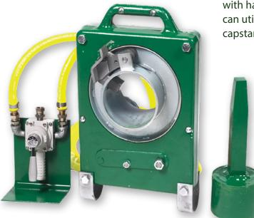
The **GO-A2** is an air-powered, hand-portable, compact Gate Opener with hand-held controls for rapid Forward-Reverse action. The **GO-A2** can utilize its capstan drive fitting, or fit over the barrel of a worn capstan and utilize the capstan's socket notches to engage the gate.
