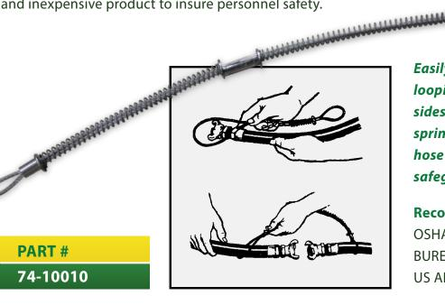
Easily installed by depressing spring and looping the wire over the hose on both sides of the connection. Release the spring and the Whipcheck locks onto the hose creating a permanent, dependable safeguard.
