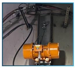
which ends or corners should be welded. A corner weld provides a perfect scenario for a weld-induced stress riser to generate a crack in the mount beam or channel, as well as in the hopper wall section to which the mount is attached.
