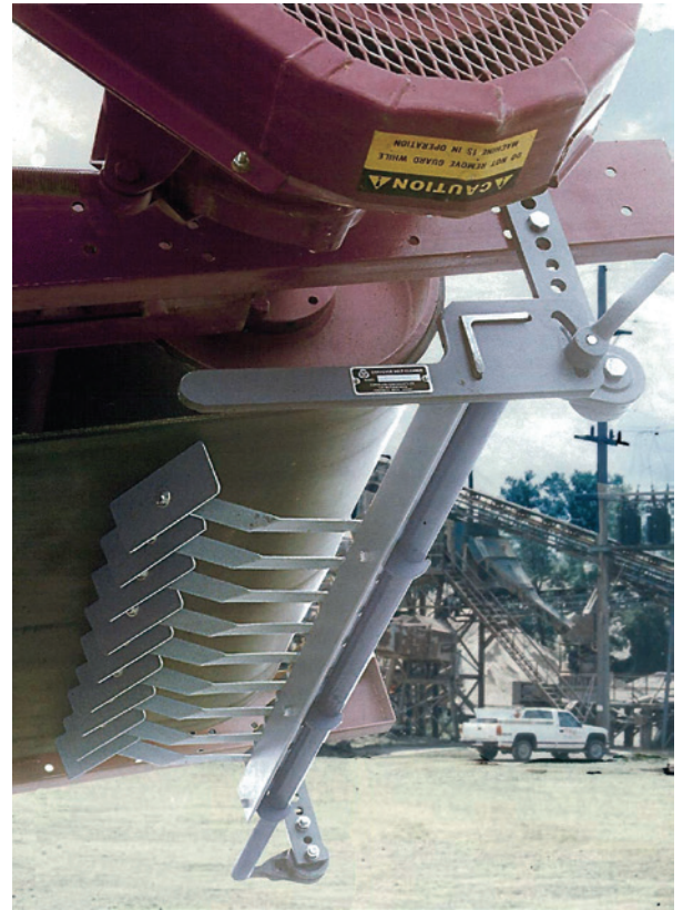
FA Belt Cleaner can be easily maintained from under the belt or through a chute door.
