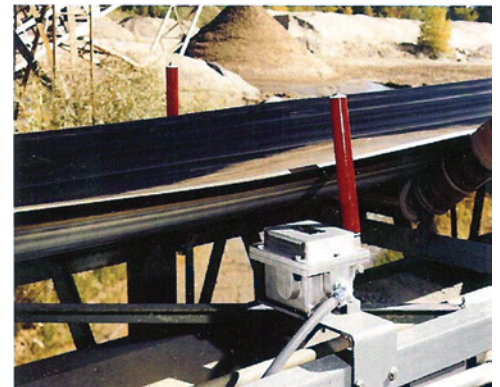
Pair of TA Conveyor Belt Alignment Switches used near head and tail pulleys.
