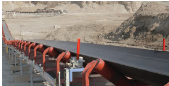
Adjustable Roller Arm set to intercept belt at its midpoint.
