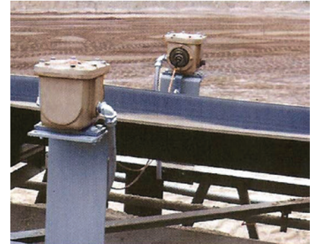
A pair of DB Damaged Belt Detectors mounted with cable underneath.
