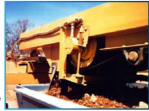
destroyed the reducers' bearings and seals. The corrosion caused the plant manager to replace the shaft-mount gear reducers every 6-9 months. Such short wear-life is a problem because it increases maintenance and downtime costs. Frequent repair also increased inventory costs and tied up valuable warehouse space because replacement gear reducers had to be kept in stock.
