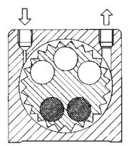
Housing made of stainless-steel Turbine wheel made of surface-hardened aluminium
