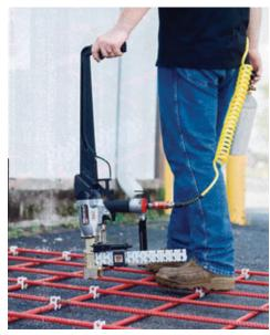
The Extension Handle's trigger is connected by a rubber-housed metal cable to the Tool's trigger to enable a worker to easily shoot the klips from an upright position - making the KODI System ideal for pour-in-place concrete construction.
