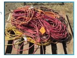
using a variety of shorter extension cords, remember the cost can escalate dramatically given the potential safety issues when making extra connections.
