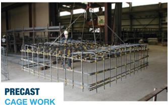
With Yellow 626 K-KLIPs, this cage is able to maintain its shape when free standing, eliminating the need for diagonal support bars and excessive wheel spacers.
